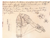
Cross-rolling process sketch of Max Mannesmann, pre 1885
