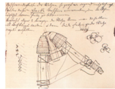
Cross-rolling process sketch of Max Mannesmann, pre 1885
